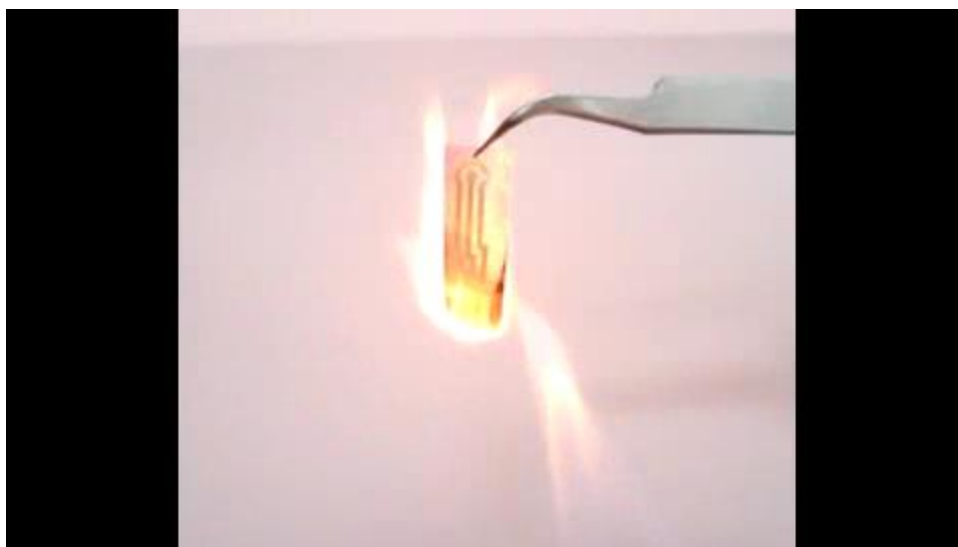
Movie S2. Captured image from supporting movie for the burnable P-paper electrode .
