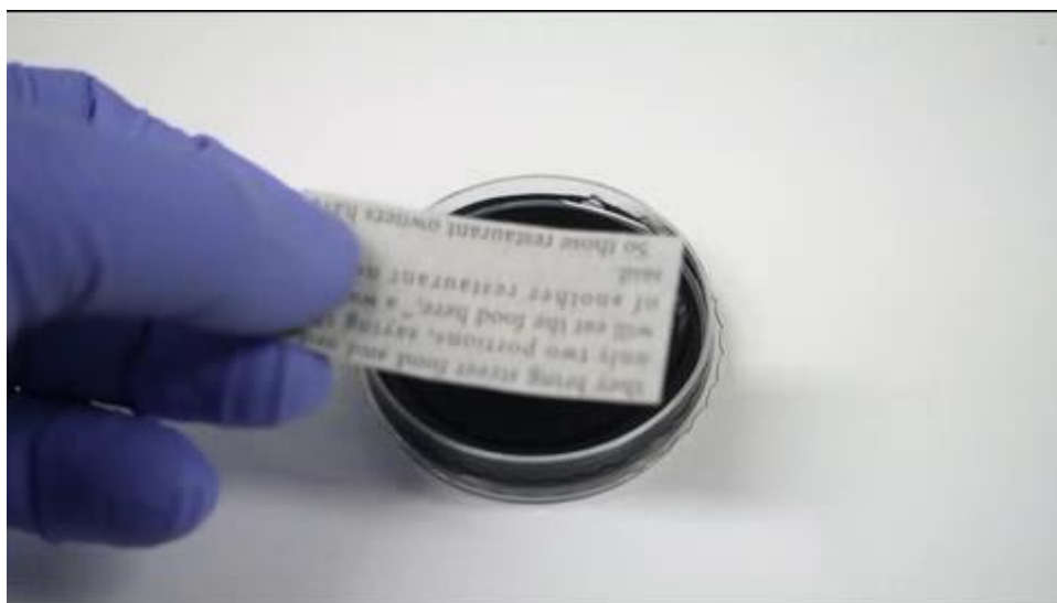
Movie S1. Captured image from supporting movie for wetting resistance of P-paper after random folding.
