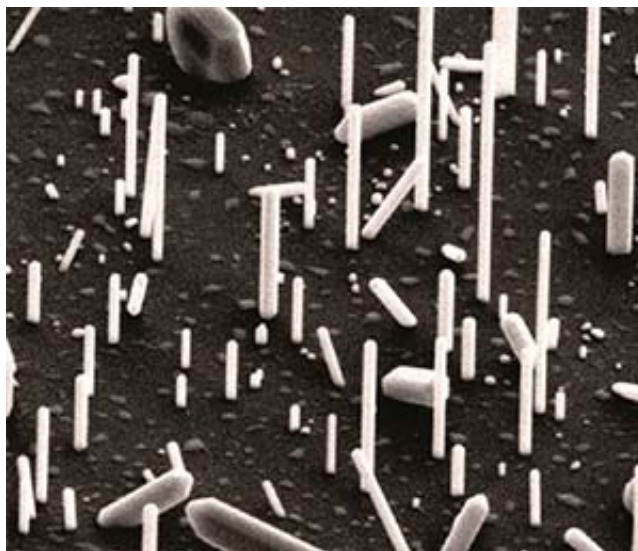
Fig. 1: Scanning electron microscopy image of vertical iron germanide nanowires grown on graphene
