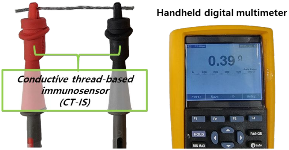
3 Figure S5. Set-up image of CT-IS using digital multimeter.
