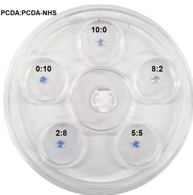
Fig. S5. Photograph of the experimental setup to detect BAs in the vapor phase using PDA-based hydrogel beads comprising. The beads were placed in a small amount of water to keep them from drying out. In this picture, cadaverine was used as an example BA.
